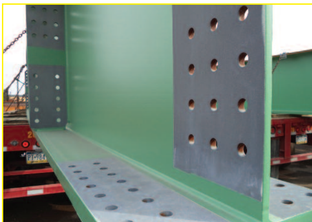
These painted girders were first metalized to increase service life.
