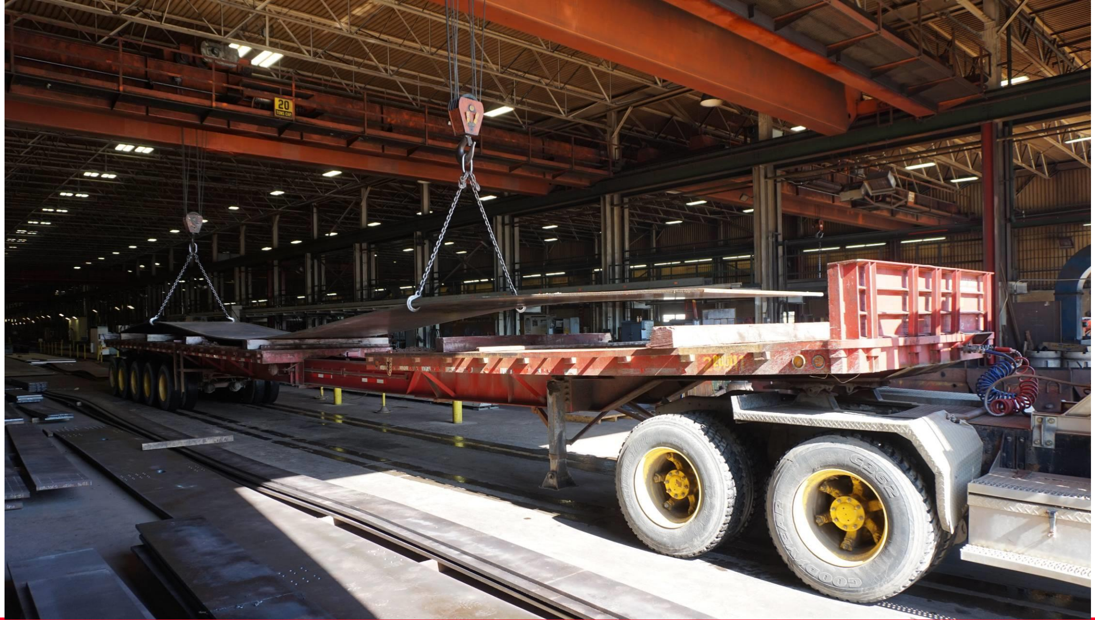
Fabrication – Hauling Plate into production bay
