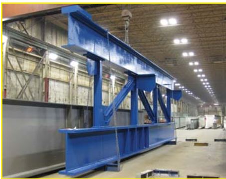
Truss chord for PSE&G project in High Steel's paint bay
