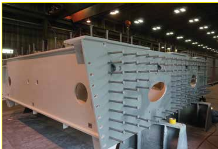
Tower Anchor box showing openings for anchor canister pipes
