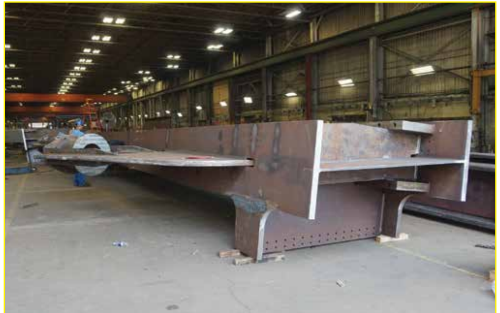
Edge girder with deck anchor in fabrication
