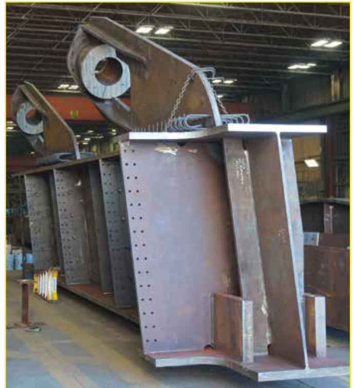
Upright edge girder showing slanted design
