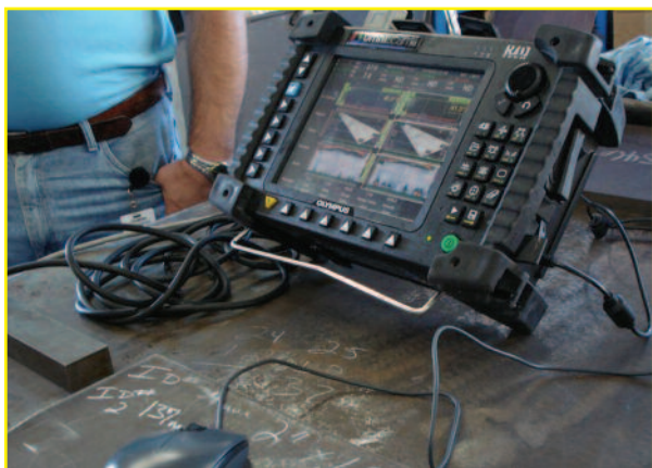
Figure 1 - This PAUT test provides six display outputs at once; as shown in the bottom two outputs, PAUT provides a picture characterization of the test.
