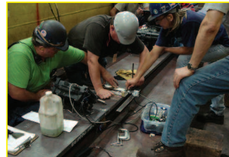
Figure 4 - High Steel's Jim Leeser, front left, Robin Dunlap, front right, and Greg Freyberg, rear left, join Shane LaPann of David NDE, front center and Olympus' Michael Moles, back right, for a phased array flange splice trial examination.
