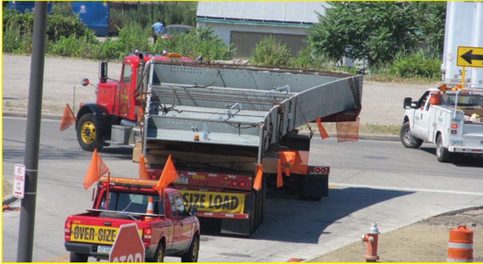
A knuckle girder is shipped from High Steel's Williamsport Plant
