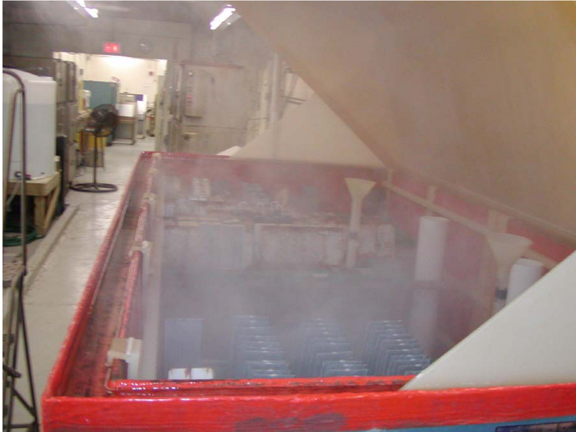
Carboline Salt Fog Machine Interior – machine opened
