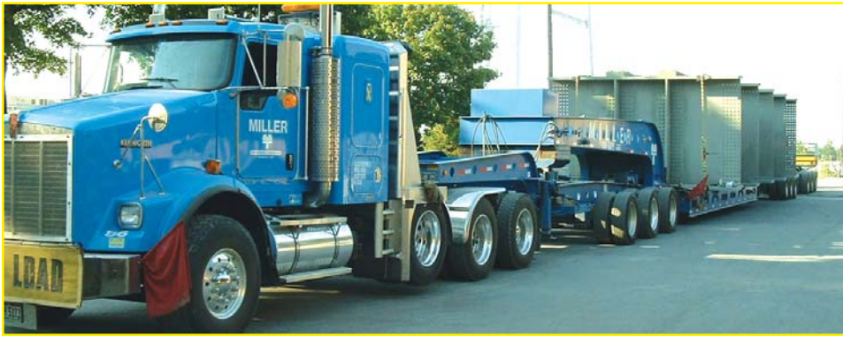
A 70-ton integral pier cap is loaded on special equipment for shipping to the job site.
