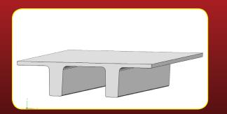
**"F" or "Form" Beam** The top flange creates a form for the deck pour
