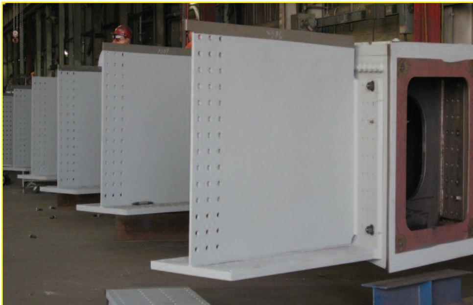
One of the project's two steel box beams with stub girders attached
